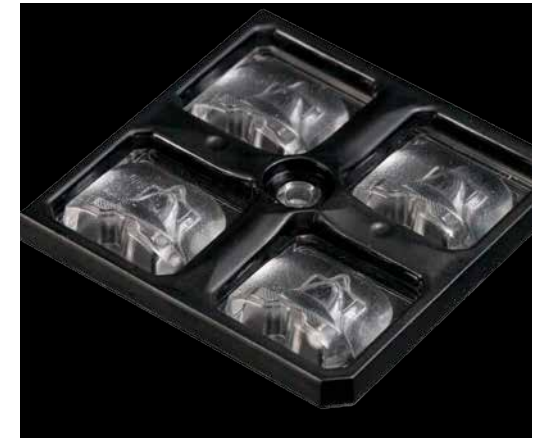
STRADA-2X2S-T3 D: 50 x 50 mm H: 7,23 mm Silicone IESNA Type III Medium light distribution
