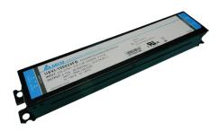
IP Rating: IP54 Max. Case Temperature: 85°CC (measured at tc-point) Lifetime: 50,000 hours @ta:45°C Power Factor : ≥0.95 Dimming Method: DALI, 1 – 254 Code for 5 - 100% Dimming range. Linear or Logarithmic variation.
