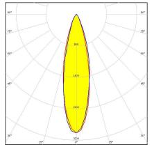
Dimensions: 67.0 mm x 67.0 mm Height: 11.10 mm ~30° medium beam
