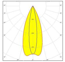
Dimensions: 67.0 mm x 67.0 mm Height: 11.10 mm  $\sim$ 40° + 20° oval beam
