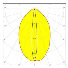
Dimensions: 33.9 mm x 33.3 mm Height: 16.90 mm 34 x 33 mm lens with ~110° x 15°
